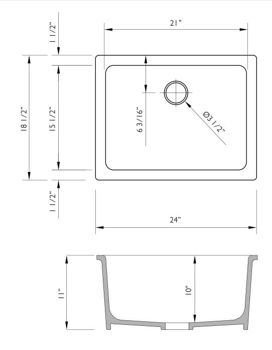
MODEL FC2418UW SIZE OUTER: 24" X 18 1/2" X 11" INNER: 21" X 15 1/2" X 10" CAPACITY (gallon) 11 WEIGHT (lbs) 64
